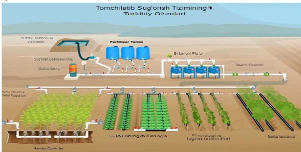
3-rasm. Tomchilab sug'orish tizimi.
